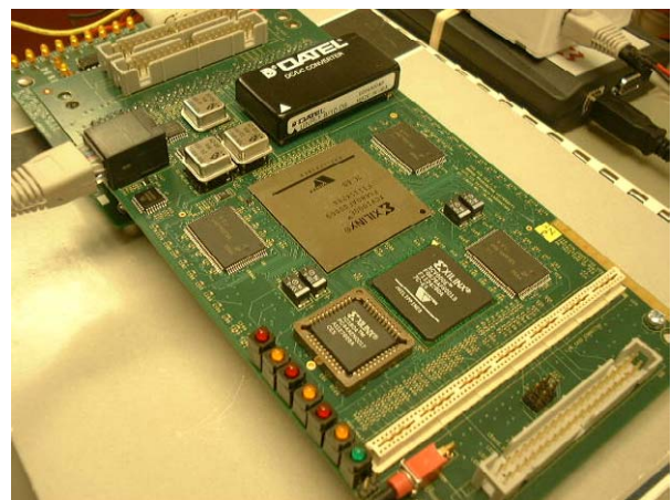
Figure 5: The FPX platform contains three SRAMs, two banks of SDRAM, two multi-Gigabit/second network interfaces, and two large FPGAs: The Reprogrammable Application Device (RAD) and the Network Interface Device (NID), implemented with a Xilinx Virtex XCV2000E and XCV600E, respectively.
